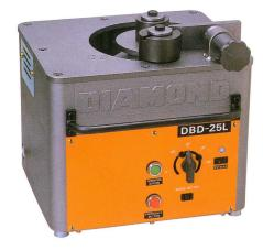
Both the DBD-25X and the smaller, lighter DBD-25L are prized field models because of their proven durability and ability to bend 25mm (1") 450N/mm² tensile strength rebars. For rebars of up to 20mm (3/4"), the DBD-19L is similarly treasured. Optional foot control, stand and bender covers are available for all three models.
